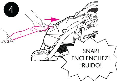
Push arm bar into hole on side of stroller.
